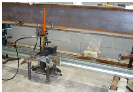
ProSigma+ Purlin from Duggan Profiles being tested. SCI used the results to produce SCI Assessed load span tables for the range of purlins.
